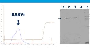
Capto Core 400 Chromatography. Blue: absorbance at 280 nm; Brown: conductivity. Western Blot of bimodal chromatography: (1) G glycoprotein VLP, (2) Concentrated flow-through fraction, (3) RABVi diafiltrate, (4) RABVi viral culture, (5) Molecular weight marker.
